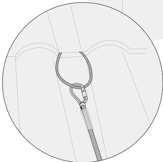
ANCHOR FOR ROOFING
